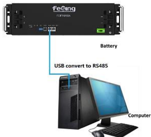
Figure 5-3: Communication Cable Connections between Battery and Computer
